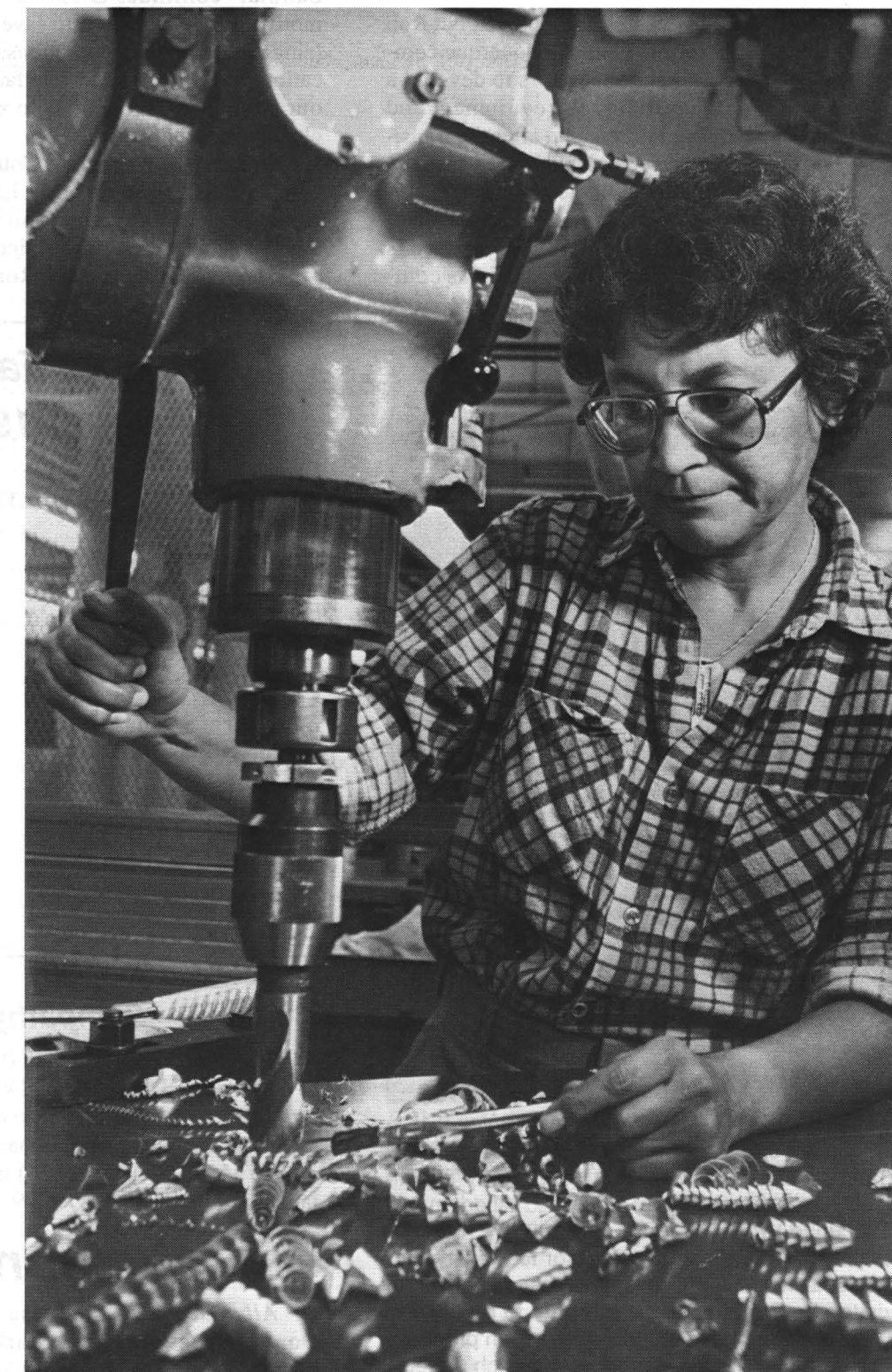
JUANITA SANCHEZ (7481) uses the Big Shop's medium-sized vertical milling machine to drill and countersink precision holes in an aluminum part.
